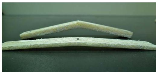
Figure 4. A single ply and a double ply ER/LC specimen after 3pb. [Color figure can be viewed in the online issue, which is available at wileyonlinelibrary.com .]
